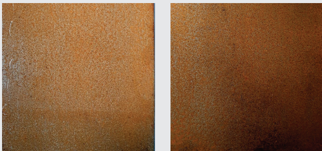
CONDITION PANEL WITH MODERATE FLASH RUST
